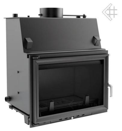
Rated power: 17 kw Average performance in water: 13 kw Diameter exag.kafsaerion: 200 CO-emission (13% O<sup>2</sup>) in%: 0.26% Water capacity: 35L Range of heat output: 8-23 Thermal efficiency: 75% Exhaust Temperature: 325 ° C
