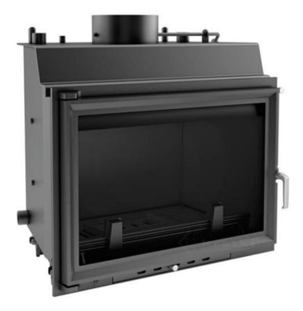
Rated power: 12kw Average performance in water: 10 kw Diameter exag.kafsaerion: 200 CO-emission (13% O<sup>2</sup>) in%: 0.69% Water capacity: 17L Range of heat output: 6-15 Thermal efficiency: 72% Exhaust Temperature: 240 ° C
