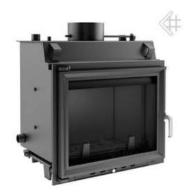
Rated power: 12 kw Average performance in water: 10kw Diameter exag.kafsaerion: 180 CO-emission (13% O<sup>2</sup>) in%: 0.29% Water capacity: 18 L Range of heat output: 6-15 Thermal efficiency: 75% Exhaust Temperature: 330 ° C
