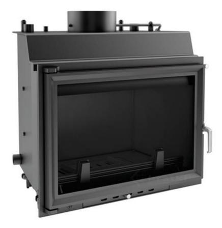
Rated power: 12kw Average performance in water: 10 kw Diameter exag.kafsaerion: 200 CO-emission (13% O<sup>2</sup>) in%: 0.69% Water capacity: 17L Range of heat output: 6-15 Thermal efficiency: 72% Exhaust Temperature: 240 ° C
