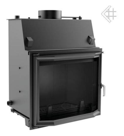
Rated power: 30kw Average performance in water: 22kw Diameter hex. exhaust: 220 CO-emission (in 13%  $O^2$ ) in%: 0.3% Water capacity: 60 L Range of heat output: 13-35 Thermal efficiency: 75% Exhaust Temperature: 315 ° C
