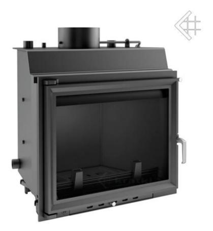
Rated power: 10kw Average performance in water: 9 kw Diameter exag.kafsaerion: 180 CO-emission (13% O<sup>2</sup>) in%: 0.69% Range of heat output: 5-13 Thermal efficiency: 72% Exhaust Temperature: 240 ° C
