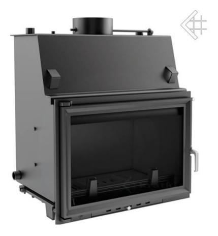
Rated power: 22kw Average performance in water: 18 kw Diameter hex. exhaust: 200 CO-emission (in 13% O<sup>2</sup>) in%: 0.3% Range of heat output: 11-29 Thermal efficiency: 75% Exhaust Temperature: 328 ° C
