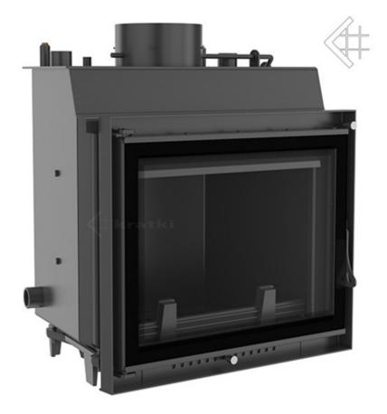
Rated power: 8 KW Average performance in water: 7kw Diameter exag.kafsaerion: 180 CO-emission (13% O<sup>2</sup>) in%: 0.69% Water Capacity: 17 L Range of heat output: 4-10 kw Thermal efficiency: 72% Exhaust Temperature: 240 ° C
