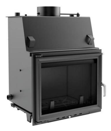
Rated power: 19kw Average performance in water: 13 kw CO-emission (in 13% O<sup>2</sup>) in%: 0.25% Water capacity: 40.5L Range of heat output: 10-24 Thermal efficiency: 75% Exhaust Temperature: 234 ° C
