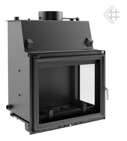
Rated power: 24kw Average performance in water: 19 kw Diameter exag.kafsaerion: 220 CO-emission (in 13% O<sup>2</sup>) in%: 0.3% Water capacity: 57 L Range of heat output: 11-30 Thermal efficiency: 78% Exhaust Temperature: 301 ° C
